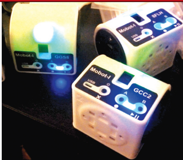
Barobo’s Mobot-I is a modular robot with body parts injection molded through Protomold, Proto Labs injection-molding service. Image courtesy of Proto Labs
