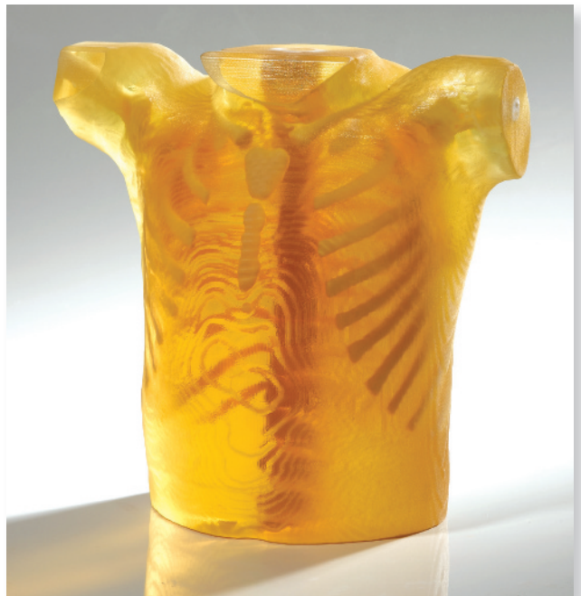
This multi-material prototype, which requires no bonding, is printed as one piece with the skeletal system on the inside (rigid white) and the exterior body printed (rigid amber). Image courtesy of GROWit LLC
